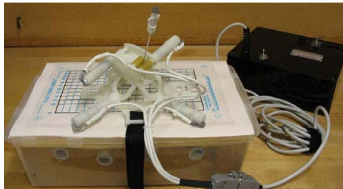
Figure 1: Beta prototype of Robopsy™ attached to a chest phantom.
