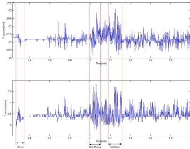
**Fig. 1** This Figure shows the noise in the position signal for a stable electromagnetic sensor on the CT scanner table measured using the ATC Flatplate transmitter. It shows the effects of taking a scout image, table movement while the gantry is running, and of actual X-ray scanning. The background noise level was observed to increase significantly when the scanner gantry was moving
