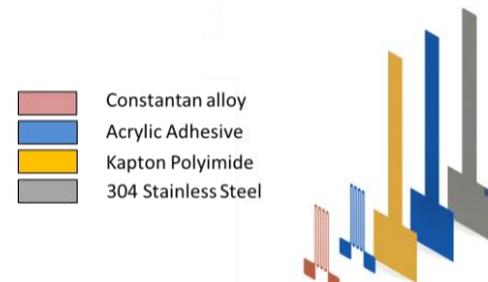
Figure 7. Gage layout on the top structural layer
