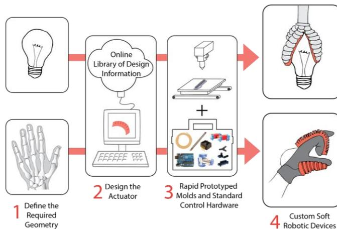
Figure 1. Envisioned design process using common virtual and physical platforms to support a range of soft robotics applications
