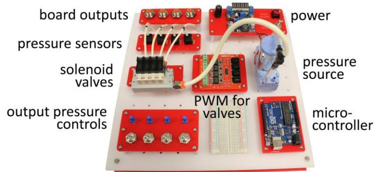
Figure 2. The Soft Robotics Toolkit website (left) and the open source hardware control board (right)
