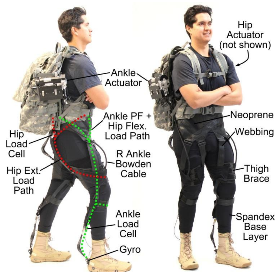
Figure 1: Load paths and components of the suit. An actuator is mounted on each side of the backpack and is connected to the suit with Bowden cables (the hip actuator is obscured). The suit includes load paths to actuate hip extension and the combination of ankle plantarflexion and hip flexion. Load cells are mounted where the Bowden cable sheaths connect to the suit, and a gyroscope is mounted on each heel.
