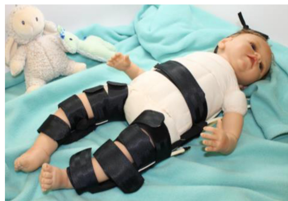
Fig. 1 Final device attached to infant mannequin showing attachment interface that holds hip and knee actuators in place
