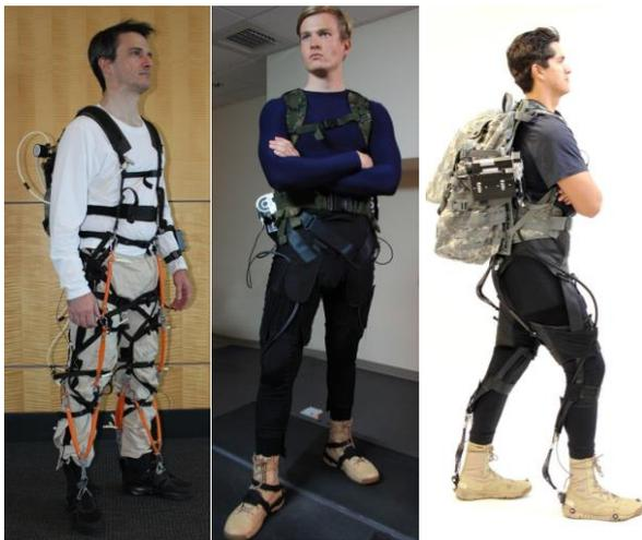
**Figure 1:** Photos of different versions of soft exosuits developed by our lab. The left suit is pneumatically-powered and was a first proof of concept; the middle is an electro-mechanical version for actuating ankle plantarflexion and hip flexion through a multiarticular suit design and on the right is a more recent version that also actuates hip extension.
