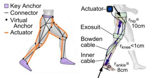
**Figure 2:** The top left diagram illustrates the concept of virtual anchors for connecting actuators to a mono-articular exosuit. The top right figures show the force distribution throughout a multi-articular suit and the moment arms at the ankle, knee and hip.
