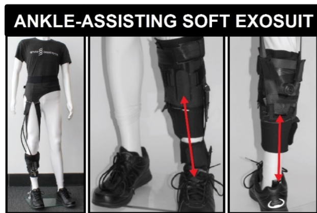
Fig 1. Assisting paretic limb propulsion and ground clearance with a soft exosuit.
