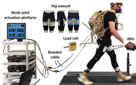
**Figure 1.** Experimental setup with a participant wearing a soft exosuit that assists hip extension via Bowden cable. The assistive force is transmitted from the multi-joint actuation platform (on the left) to the wearer.
