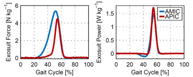
Fig. 3. (a) Average exosuit force and (b) average exosuit power for the AMIC and APIC.
