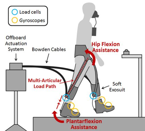
Fig. 1. Experimental setup with the offboard actuation system and the multi-articular soft exosuit that assists with both ankle plantarflexion and hip flexion
