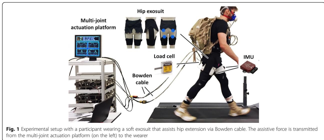
our previously described hip soft exosuit [28], the components used for this study were constructed with a woven fabric with reinforcement webbing and neoprene was added to the waist belt close to where it interfaced to the iliac crest of the wearer. The multi-joint actuation platform was a tethered system designed to provide biologically inspired torques to multiple joints through Bowden cables either individually or simultaneously [44].
