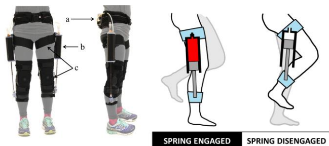
Fig. 1. Left: (a) control system, (b) air spring, (c) fabric interface. Right: during early stance phase, a solenoid valve seals the air chamber and restricts flexion. When opposite heel strike is detected, the valve opens and the knee can flex freely.
