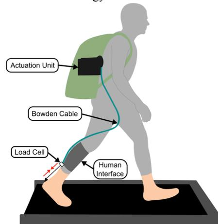
**Figure 1.** Test setup for treadmill walking trials where a mobile actuation unit mounted on a backpack generated force and Bowden cables were used to transmit that force to the shank interface.
