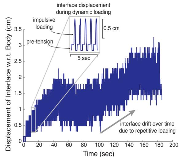
**Figure 2.** Interface displacement with respect to the body vs. time, as a result of repetitive impulsive loading. Interface migration (slippage) is evidenced by the shifting of the baseline displacement on a longer time scale. Inset: displacement during dynamic loading is seen on a shorter time scale, where the interface displaces temporarily and then recoils back to the same position.
