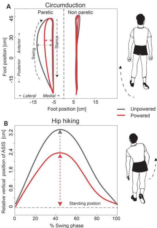
**Figure 2:** Compensatory gait pattern of representative subject showing **A.** Circumduction and **B.** Hip Hiking during exosuit unpowered and powered conditions
