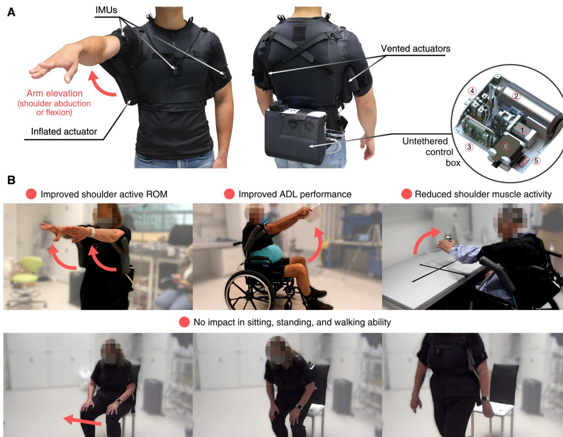
Fig. 1. Untethered, portable soft robotic wearable for shoulder monitoring and assistance. (A) Shown are the main robotic components of the robotic wearable shirt. Two textile-based soft actuators, anchored under the armpits, provide dynamic assistance while inflating. To assess user movement ability and assist the shoulder in an intuitive way, three inertial measurement units (IMUs), placed on the torso and both upper arms, estimate upper limb kinematics. A control box, anchored to the waist of the user (total weight, ~3.6 kg), powers the robotic wearable and runs the gravity compensation strategy. Textile components include strap-based adjustments for optimal fit. Arm elevation is defined as either shoulder abduction or shoulder flexion. Other upper limb movements, such as shoulder horizontal flexion, are not restricted. The user can actively control their motion by leveraging any residual strength or capacity as the robotic wearable helps to compensate for the effects of gravity. Control box components: (1) scroll compressor, (2) 750-ml air reservoir, (3) microcontroller and custom electronics, (4) proportional valves and custom manifold, (5) electronic speed controller, and (6) batteries. (B) Study participants with ALS performed a series of activities from the study protocol, including shoulder abduction and flexion, holding an object, and the 6-min walk test. Red arrows indicate direction of movement. ROM, range of motion; ADLs, activities of daily living.
