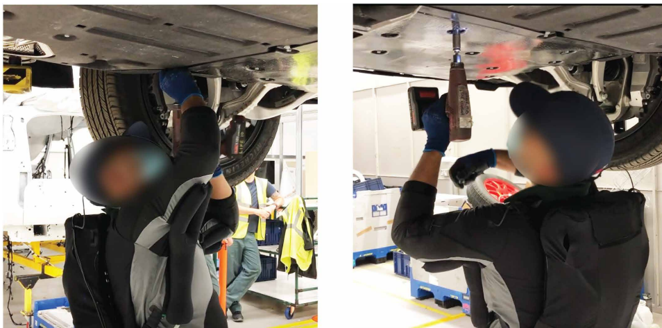
Fig. 7. Factory worker performing overhead tasks while assisted by the robot.
