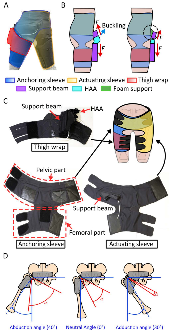
Fig. 3. Design principles: A) a picture of the device with three different components: an anchoring sleeve, an actuating sleeve, and a thigh wrap; B) a schematic figure describing a role of the wedge-shaped foam piece to prevent from outward expansion; C) detailed three components: first, the anchoring sleeve (blue) is tightened around the hip, and then the actuating sleeve (yellow) and the thigh wrap (red) anchor to the anchoring sleeve via hoop and loop fasteners; D) the actuator angle ( \alpha ) requirement at neutral angle of 0^\circ . The support beam is attached on the femur. The support beam moves with the same angle in the frontal plane as hip ab/adduction angle. The minimum actuator angle relates to the maximum adduction angle.
