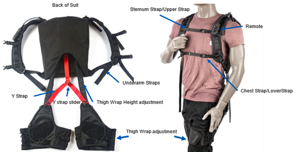
Fig. 1. Verve SafeLIFT exosuit, which includes the actuated ribbon (Y-Strap), adjustable components, remote to control actuation strategies, and depiction of the chest/sternum straps.
