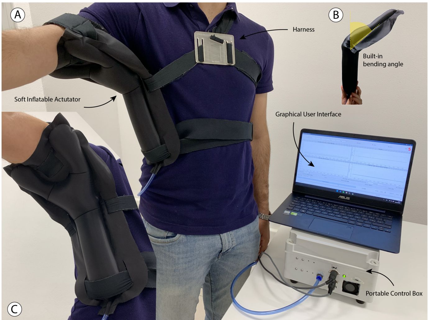
Fig. 1. A) Overview of our soft wearable robot for shoulder assistance. It consists of a single-layer inflatable actuator, a custom harness (total weight of harness and actuator, 265g), a portable (2.1kg) benchtop control box, and a graphical user interface. The shoulder device is unilateral but can be mounted on either side of the body. (B) A close-up of the actuator and its characteristic Y-shape for improved comfort. (C) Demonstration of the built-in 45 degrees bending angle of the soft actuator. This angle is meant for better fitting under the armpit and thus improved torque transferring.
