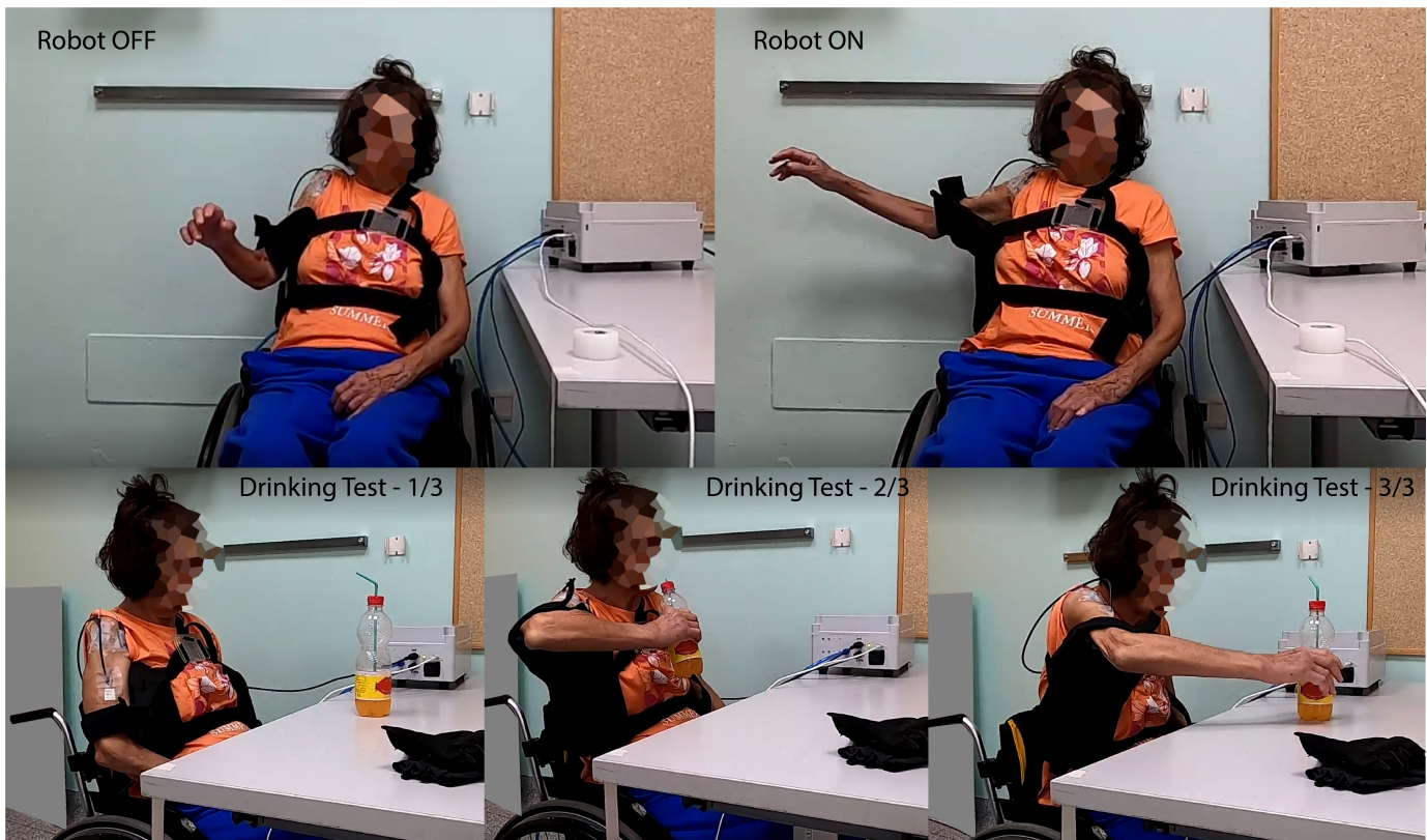
Fig. 10. Participant P12 performing the lift and hold test in the two conditions, robot OFF vs robot ON (top pics). The improved workspace allowed the same participant to drink from a bottle, a task not achievable without the robot (bottom pics).
