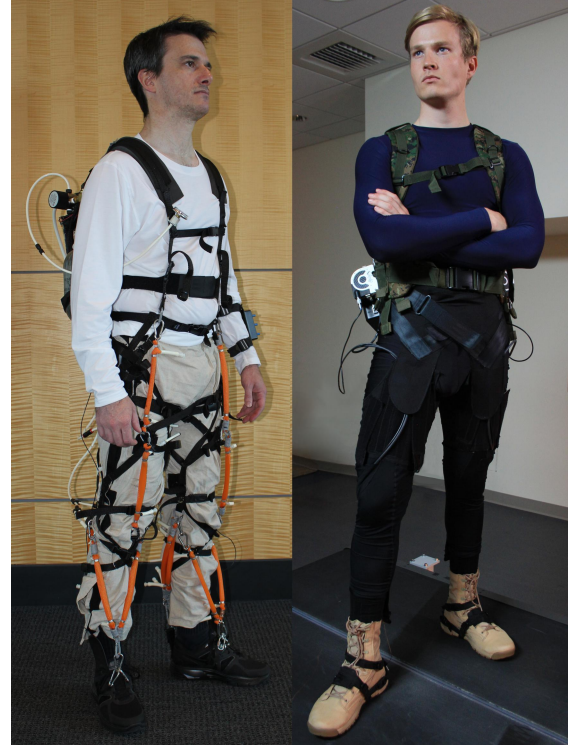
Fig. 1. Photos of two soft exosuits developed by our lab. The left suit is an early pneumatically-powered design that controls each of the joints in the leg in both directions in the sagittal plane. The right suit is our latest multi-articular design aiding ankle plantarflexion and hip flexion, and is actuated by geared motors driving Bowden cables.
