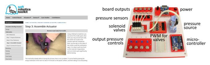
Figure 2. The Soft Robotics Toolkit website (left) and the open source hardware control board (right)
