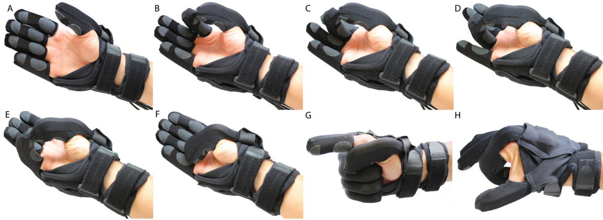
Figure. 9. Range of motion of the soft robotic glove. A. Pretension of the fabric sleeves surrounding the fiber-reinforced actuators offers full hand extension. B-F. Executing the Kapandji test [21] with the soft robotic glove for thumb range of motion. G. Finger flexion with index finger straight. H. Index finger flexion.
