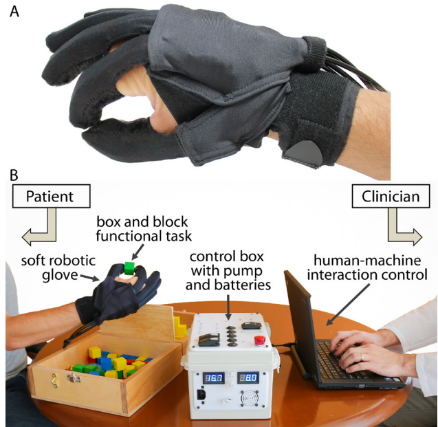
Figure 1. A. The prototyped hydraulically actuated soft robotic glove. B. Patient-clinician setup that utilizes the soft robotic glove to perform hand rehabilitation scenarios.
