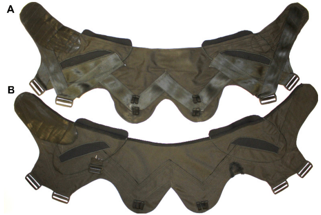
FIGURE 4. THE TWO PROTOTYPES OF THE WAIST BELT EVALUATED IN THIS PAPER INCLUDING (A) WEBBING-REINFORCED WAIST BELT AND (B) WEATHERMAX-REINFORCED WAIST BELT.
