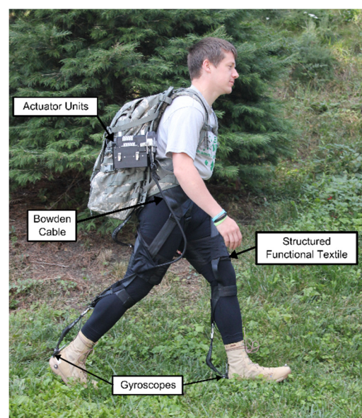
FIGURE 1. OVERVIEW OF THE SOFT EXOSUIT SYSTEM INCLUDING ACTUATOR UNITS, BOWDEN CABLES, STRUCTURED FUNCTIONAL TEXTILE, AND GYROSCOPES.
