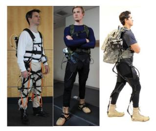
Figure 1: Photos of different versions of soft exosuits developed by our lab. The left suit is pneumatically-powered and was a first proof of concept; the middle is an electro-mechanical version for actuating ankle plantarflexion and hip flexion through a multiarticular suit design and on the right is a more recent version that also actuates hip extenson.
