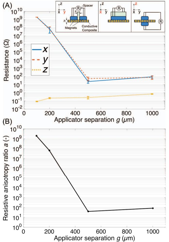
Fig. 2. Characterization of resistance of fabricated composite samples. (A) In-plane ( $x$  and  $y$ ) and through-thickness ( $z$ ) resistances as a function applicator separation  $g$  (average of four measurements, error bars are  $\pm$  one standard deviation). Inset, schematic depiction of the experimental setup. (B) Ratio of the mean of the average in-plane resistances to through-thickness resistance,  $a$ , against applicator separation  $g$ .
