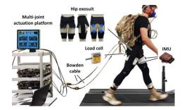
**Figure 1**. Experimental setup with a participant wearing a soft exosuit that assists hip extension via Bowden cable. The assistive force is transmitted from the multi-joint actuation platform (on the left) to the wearer.
