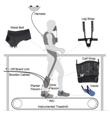
Figure 1: Experimental setup and exosuit components
