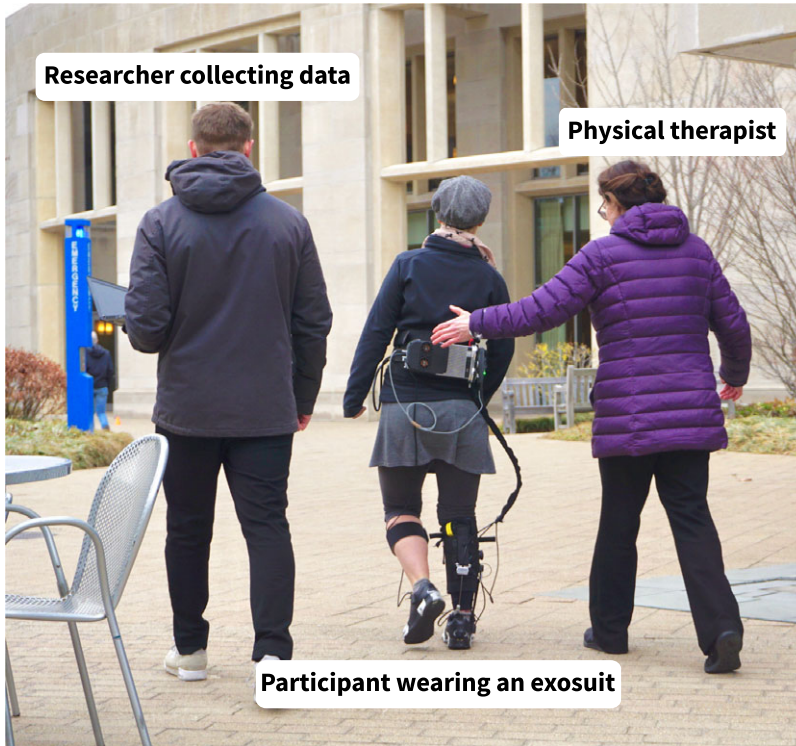
Figure 6. Experimental setup for collecting gait metric data during community-based walking. The participant was guided by a physical therapist for a total of five laps around a well-trafficked plaza at Harvard University. Sensor data were streamed via Bluetooth to a nearby computer, carried by a researcher following the participant.
