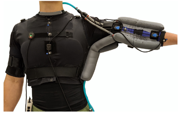
Fig. 1. The worn element of the multi-joint soft wearable robot is comprised of two main components, a shoulder component and a newly developed elbow component. The robot is powered and controlled by an external fluidic supply, and uses 3 inertial measurement units to measure the current pose of the assisted limb for control feedback purposes.
