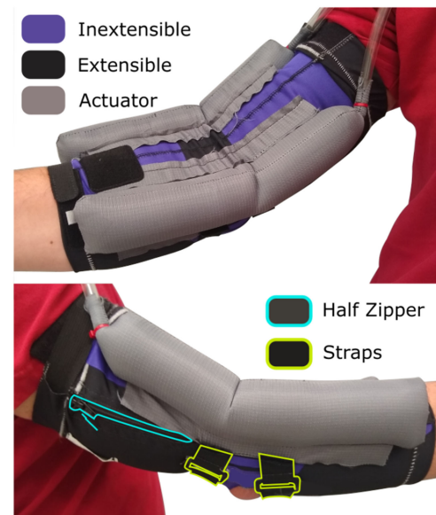
Fig. 2. The structure and manufacture of the soft wearable elbow component is similar to that of the shoulder component. It combines inextensible textiles with extensible ones to securely anchor the actuators while remaining comfortable. The included straps allow for size adjustment to ensure appropriate fit.
