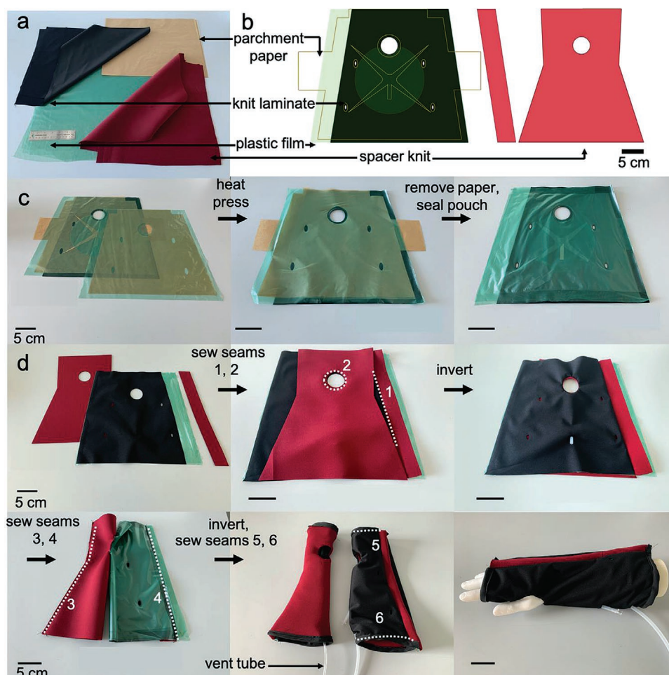
Figure 2. Fabrication process. a) Photograph of sheets of materials used in fabrication of the FFC. b) Schematic diagram of the pattern used to laser cut these materials. c) Photographs of the cast at various stages of the fabrication process. Heat pressing, with patterns of parchment paper as sacrificial layers, is used to fabricate the thermoplastic pouch and fluidic channels for the foam. The red fabric pieces are sewn to the black fabric containing the green pouch (seams 1 and 2). The red fabric is then inverted through the thumbhole and seams 3 and 4 are sewn. Finally, the garment is inverted again, and the top and bottom seams (5 and 6) complete the fabrication process. A more detailed figure describing the fabrication process can be found in Figure S1 in the Supporting Information.
