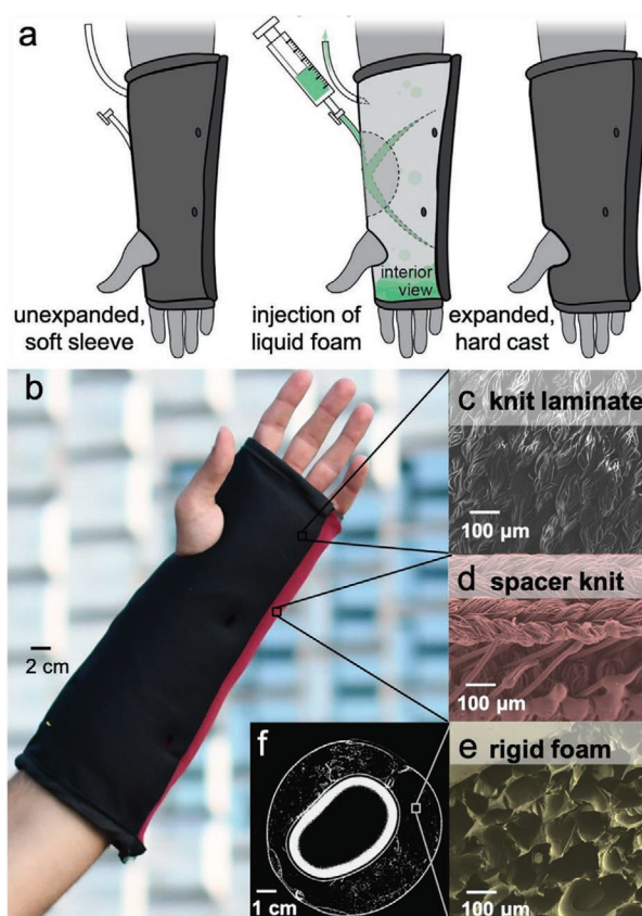
Figure 1. The expanding foam-fabric cast (FFC). a) A schematic diagram describing the application process. b) A photograph showing the expanded FFC on a wrist. Scanning electron microscope (SEM) images showing c) the knit laminate, d) the spacer knit fabric, and e) the rigid foam. SEM images are false colored to reflect the colors of the respective materials. f) A transverse section of the cast obtained from X-ray computed tomography.
