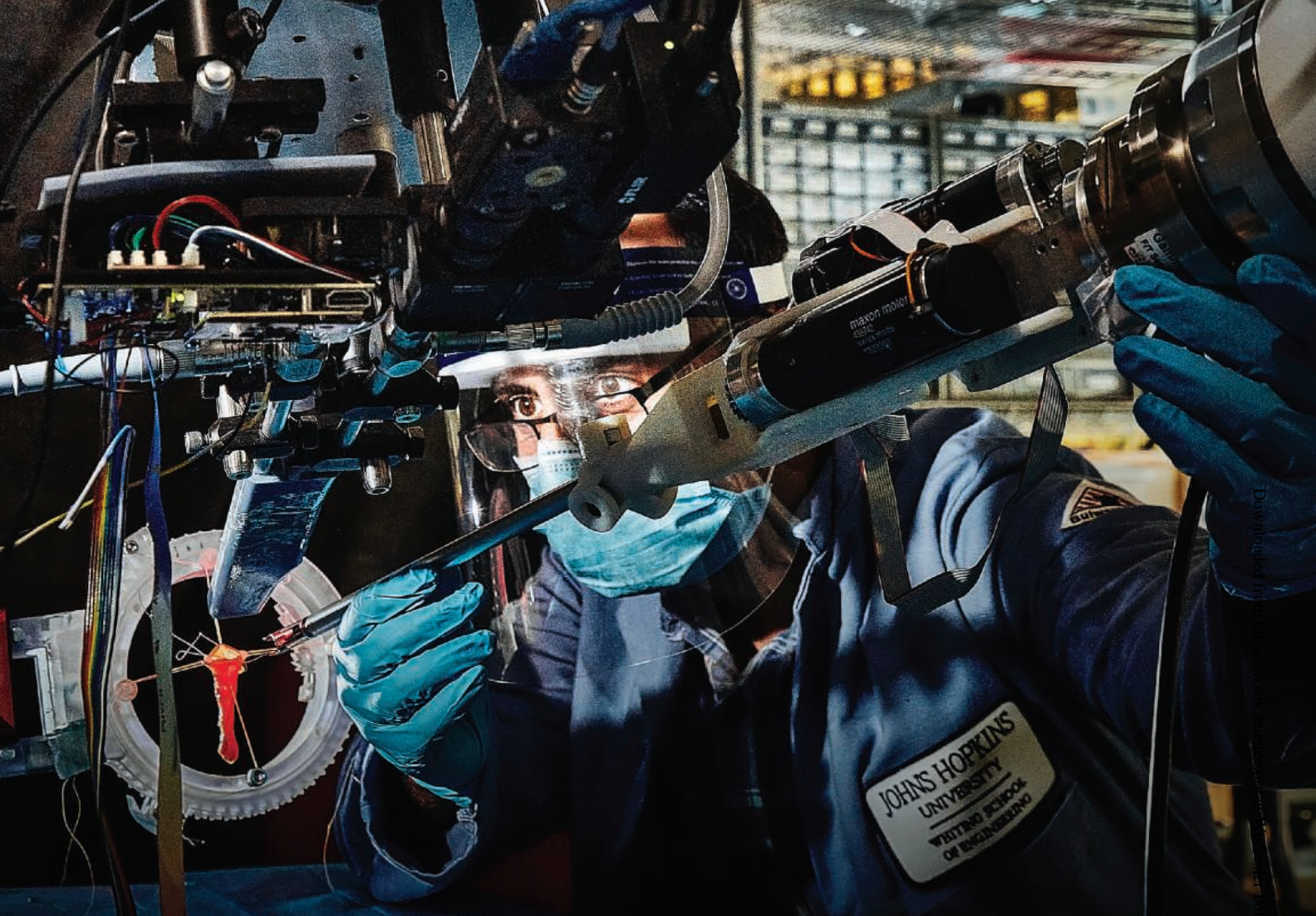
The Smart Tissue Autonomous Robot (STAR), which is holding a needle driver, needle, and suture in preparation for suturing intestinal tissues, is inspected.
